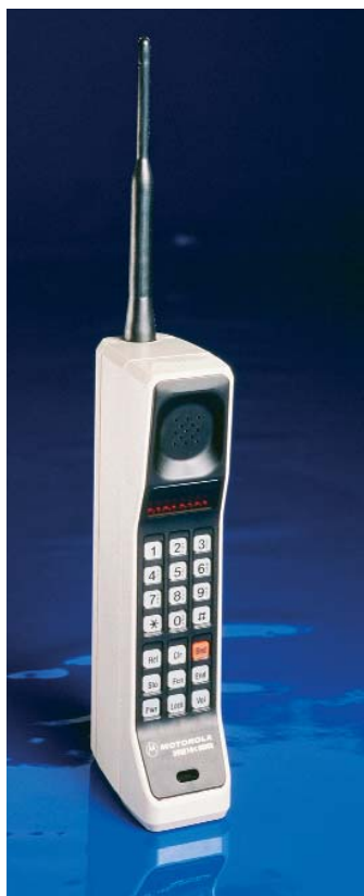
The Motorola Dyna-TAC from 1983 was the first handheld cellular phone (from: http://www.motorola.com/mediacenter/graphics/ )
